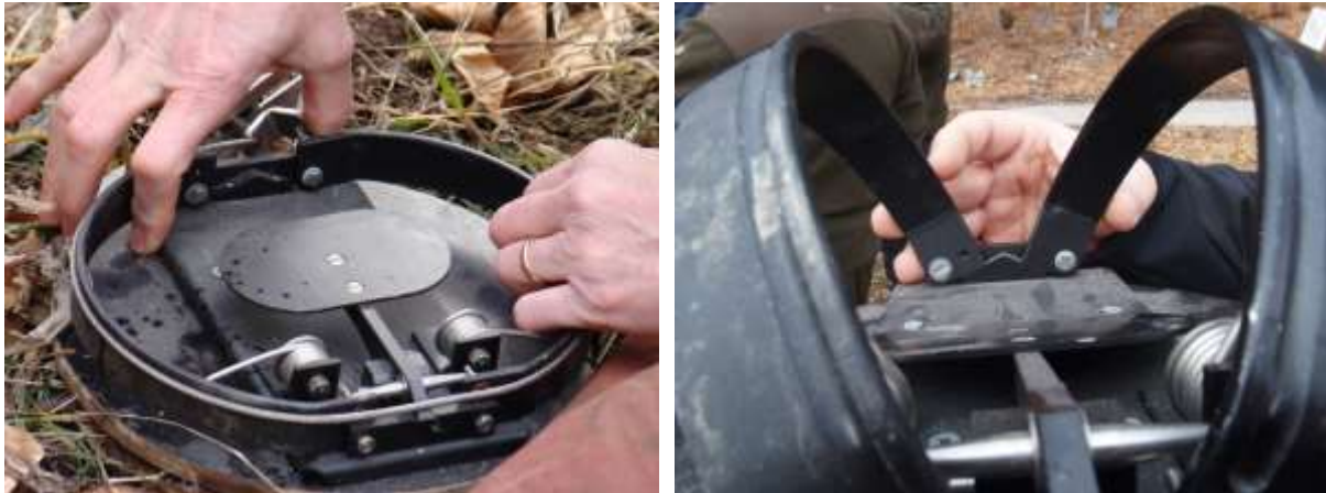
Fig. 2 Snare traps developed and recommended by KORA to be used at kill sites
